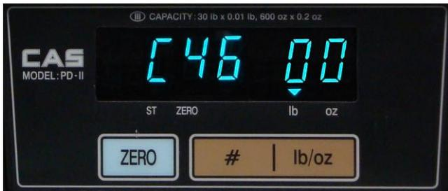
19. The scale should display “C46 00”. If it does not, use the # button to move the cursor and the lb/oz button to change the value.
