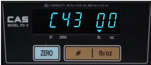
13. The scale should display “C43 00”. If it does not, use the # button to move the cursor and the lb/oz button to change the value.
