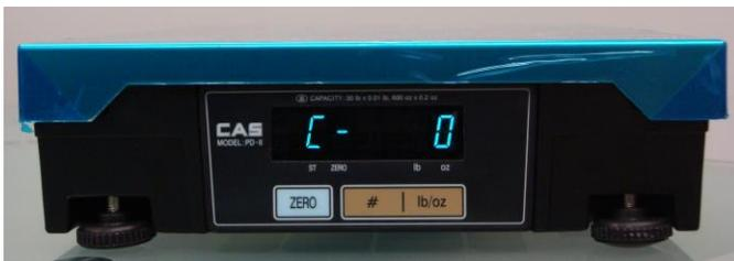
21. The scale should display “C-4”. Press the lb/oz button until it displays “C-0”.
