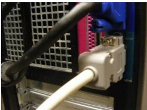
2. Plug the serial cable connected to the scale into the port.
