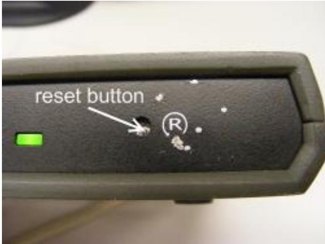
1. Press the reset button on the LS6000 (right side of the front) while holding down the **Summary** button on the KVS.
