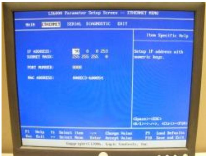
3. Select **In Progress** on the Bump Bar until **ETHERNET** is highlighted on the monitor.
